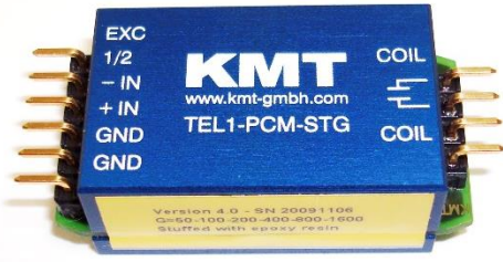
New version 4.0 without external CAL pins
