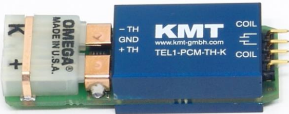
with female K type thermocouple connector
